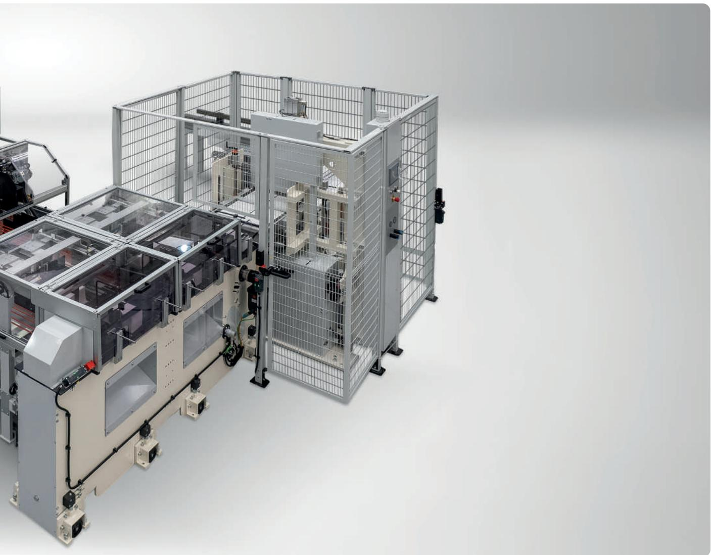
The line is equipped with modular folding plates for  $\frac{1}{2}$  or  $\frac{1}{4}$  folded napkins, to meet the specific requests of each customer in terms of configuration and type of product.
