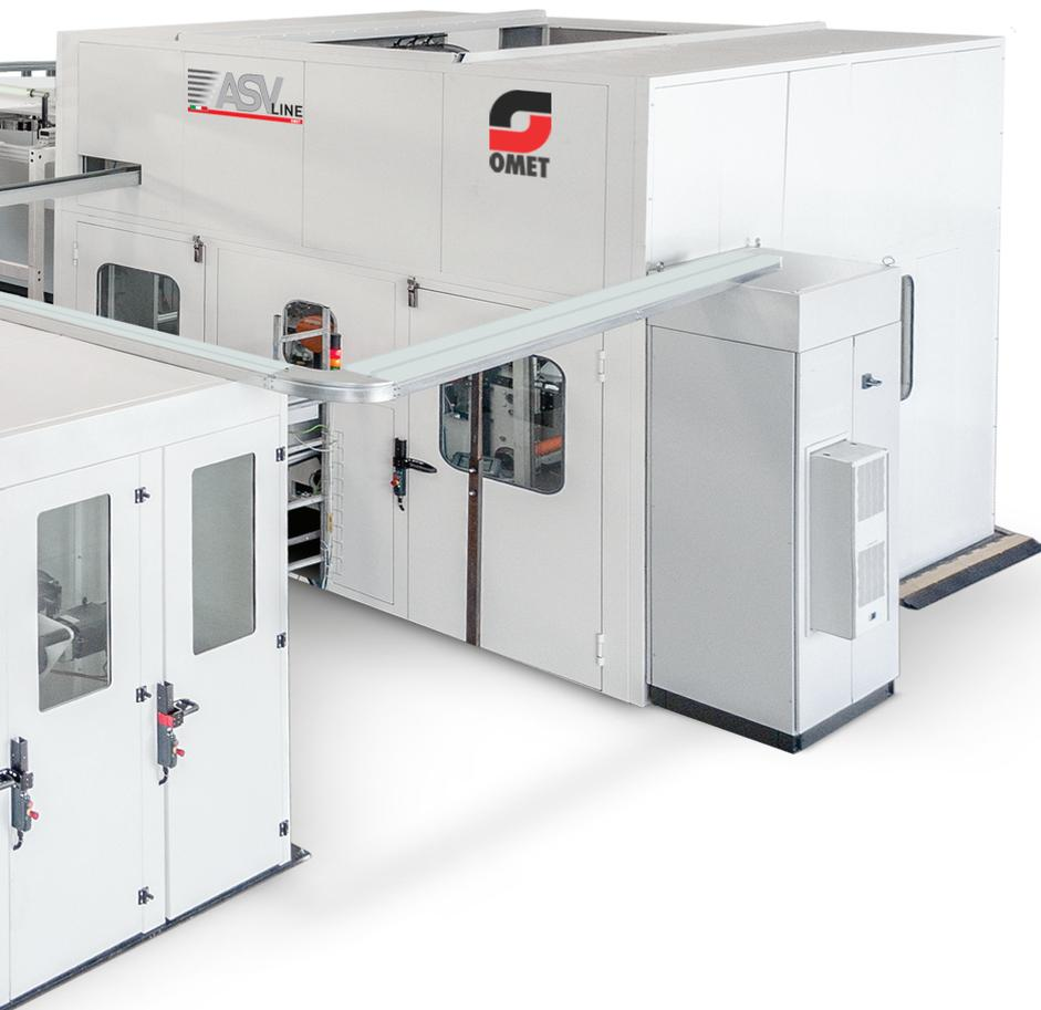
The ASV Line is the automatic interfolding line specially developed by OMET for the production of interfolded towels, kitchen paper, facial tissue and toilet paper, which guarantees a flexible and efficient production process. Thanks to the latest technologies implemented on the ASV Line, the machine is fully automatic and automated and easy to use for the op-
